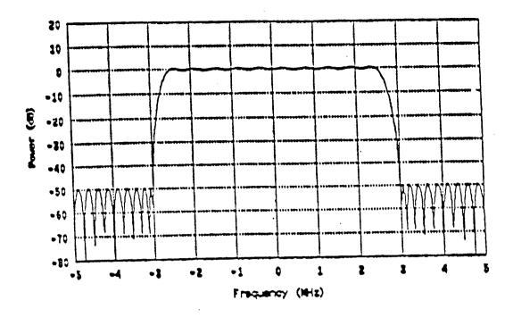
Figure 6: Spectral Shaping Filter Frequency Response
