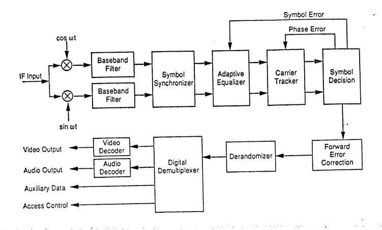
Figure 3: Demodulator Components
