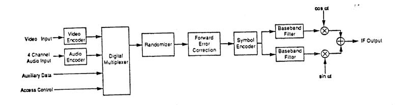
Figure 2: Modulator Components
